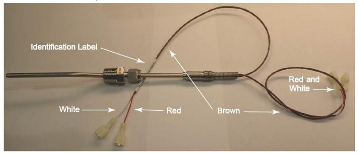
EEG and LVG vat replacement kits P/N: 140206, 140207, 140208, 140209, 140289, 140599, 140601 will continue to have one high limit thermocouple probe for full vats and two for split vats.
